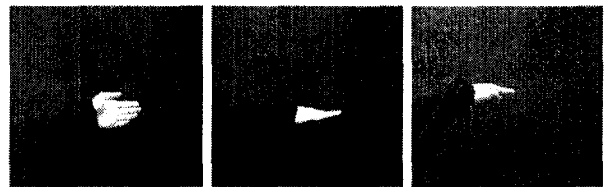
Figure 5: Control level gesture (left), transition level gesture (middle) and gripping gesture (right).
