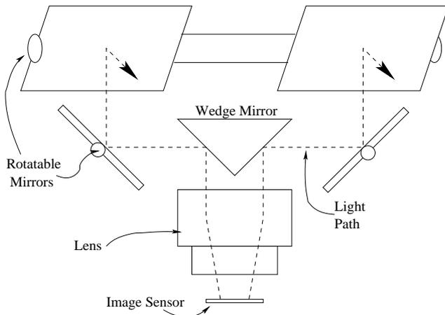
Figure 4: Mirror Based Optical System
